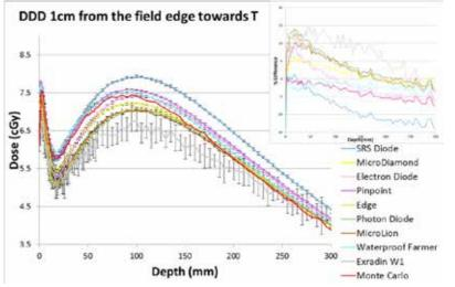
Figure 1: Comparison between MC-calculated and measured divergent depth doses 1cm from the field edge
